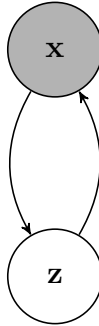
Figure 1: A graphical representation of the VAE architecture where \mathbf{x} is the content (image) of size D and \mathbf{z} its latent representation (code) of size d \ll D .
